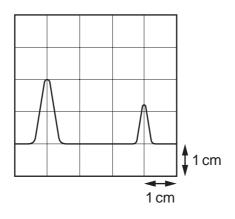
The pulse takes  $6.3\,\mu\text{s}$  to travel from the transmitter to the reflector.
